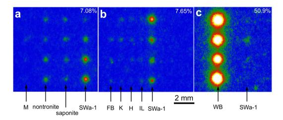
**Figure 2.** Read-out images of IPs covering the substrates with (a) several smectite species, (b) ferruginous smectite (SWa-1) and several mineral species other than smectite, (c) WB and SWa-1. Four particles were arranged on the substrates for each mineral species. The radioactivity input to the solution was 1.85 Bq and the reaction period was 24 hours. The meanings of the figure at the top-right of each image and abbreviations of the minerals are the same as those in Fig. 1.
