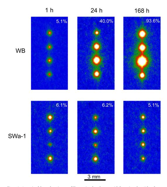
Figure 3. A matrix of the read-out images of IPs covering the substrates with four mineral particles of (top) WB and (bottom) SWa-1, reacted with 1.85 Bq <sup>137</sup>Cs solution for various periods. Notice that only one mineral species was placed on the substrates and the mineral particles were different for each run.
